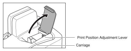
**2** While squeezing in both sides of the print position adjustment lever, move the print cartridge carriage up or down to adjust the print position.
